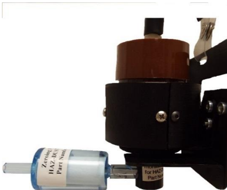
Figure 3-13. Zeroing filter (p/n ZA-7204) being attached to the Thoracic sampling inlet.
