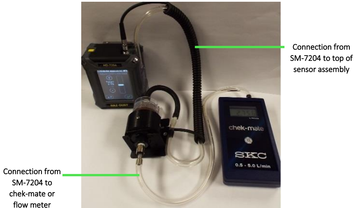
Figure 3-12. Connecting SM-7204 to SKC chek-mate
