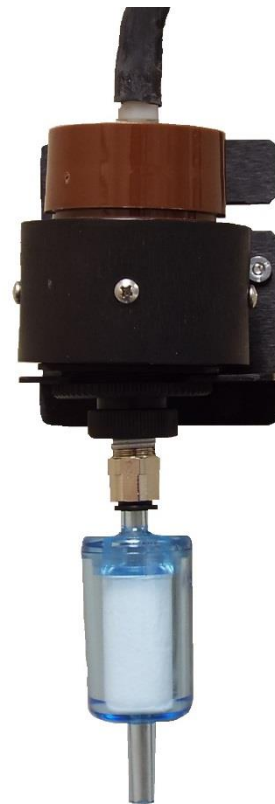
Figure 3-14. Zeroing filter (p/n ZA-7204) attached to the IOM Inlet.
