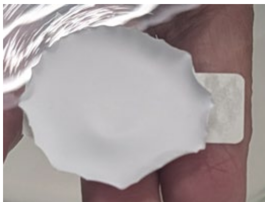
Figure 1. PVC filter exposed to 70 C (158 F)
