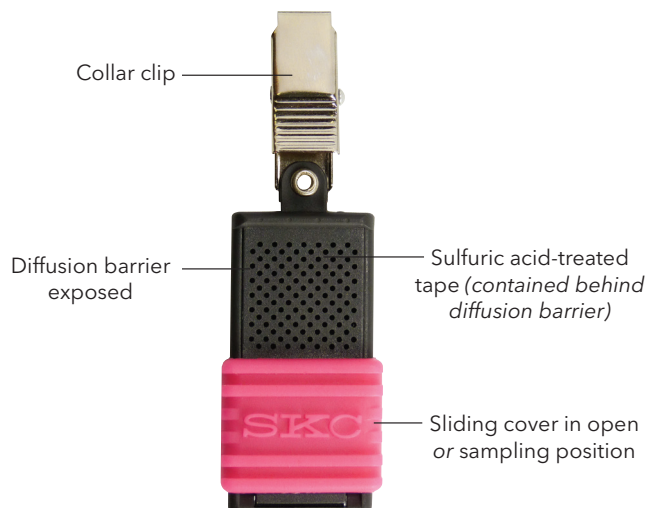
UME x 300 Sampler with sliding cover in sampling position
