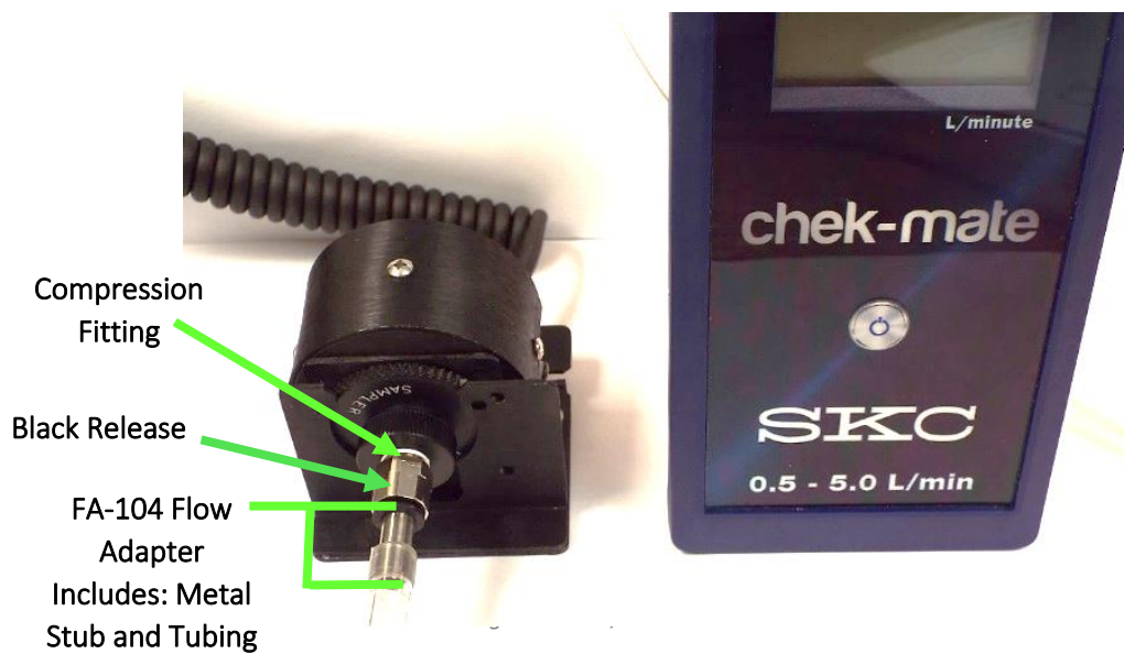
Figure 3-11. P/N FA-104 Inserted into Sensor
