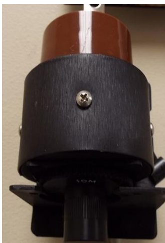
Figure 3-15. CS-7204 being inserted into HD-7204 sensor
