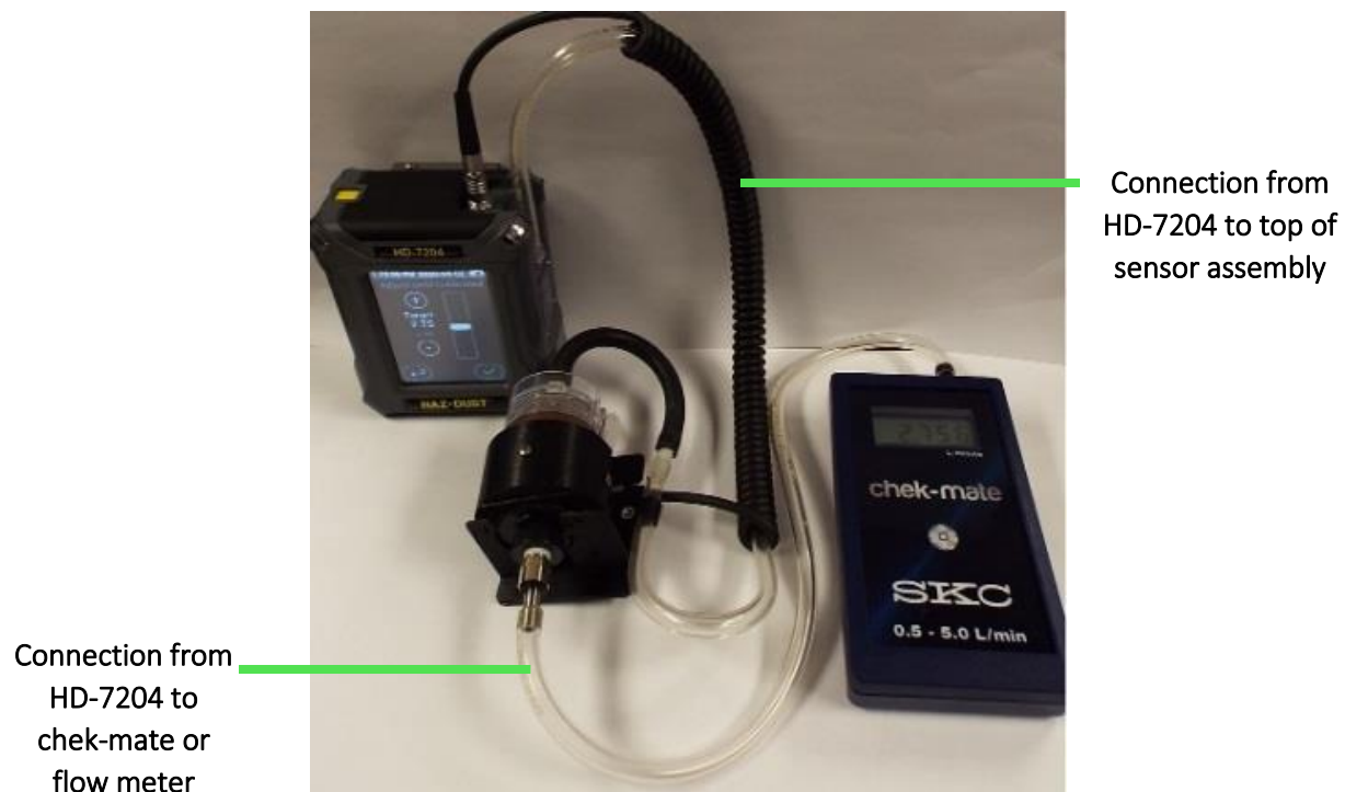
Figure 3-12. Connecting HD-7204 to SKC chek-mate
