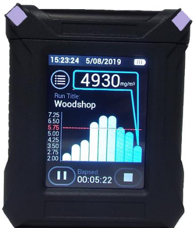
Figure 3-16. Flow Faults cause purple lights to flash
