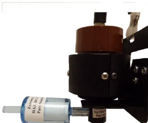
Figure 3-13. Zeroing filter (p/n ZF-102) being attached to the Thoracic sampling inlet.
