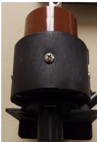
Figure 5-1. CS-7204 being inserted into HD-7204 sensor
