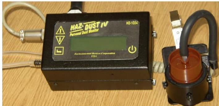
Figure 1-1. Picture of the Haz-Dust IV.
