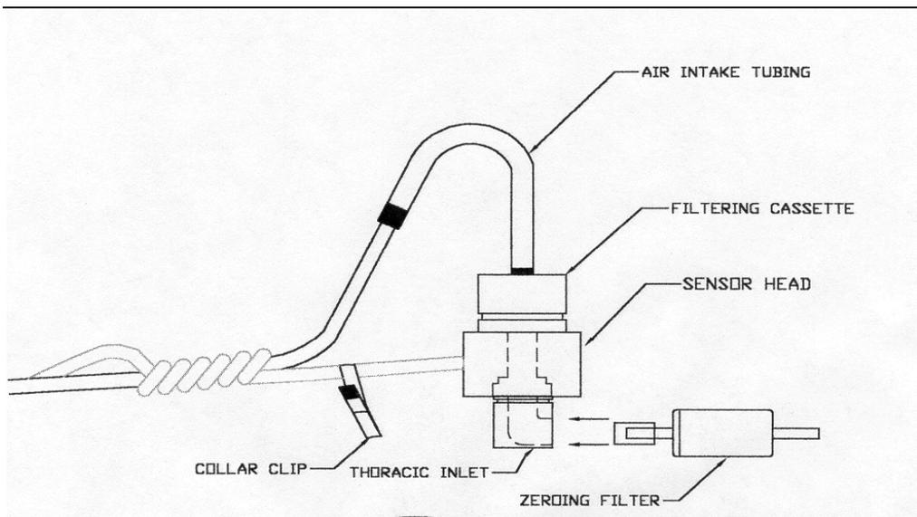
Figure 3-6. Diagram of zeroing filter being inserted into the Thoracic sampling inlet. This procedure is used for both Thoracic and Inhalable dust particles.
