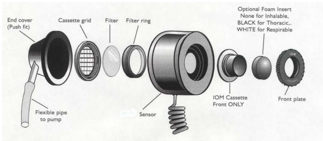
Figure 3-5. Disassembled IOM Sampling Adapter. SKC catalog number 225-70.
