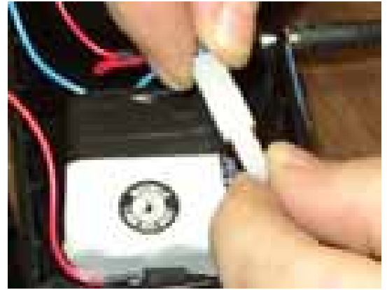
Figure 2B: Reconnect battery from nylon connectors. NOTE: DO NOT PULL ON WIRES.
