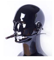
The Face Level Sampling Headset was developed in a research project partly funded by the Swedish Work Environment Authority and carried out at Stockholm University, Sweden.
