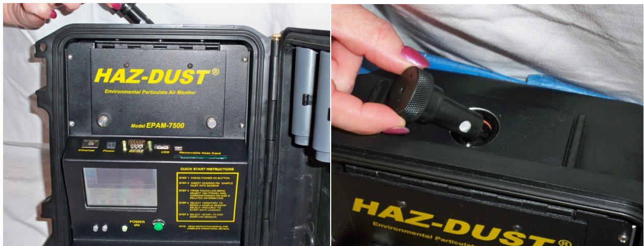
Figure 5-1. Inserting CS-105 into Haz-Dust Sensor.
