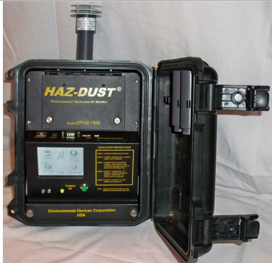
Figure 1.2. Picture of the Haz-Dust EPAM-7500
