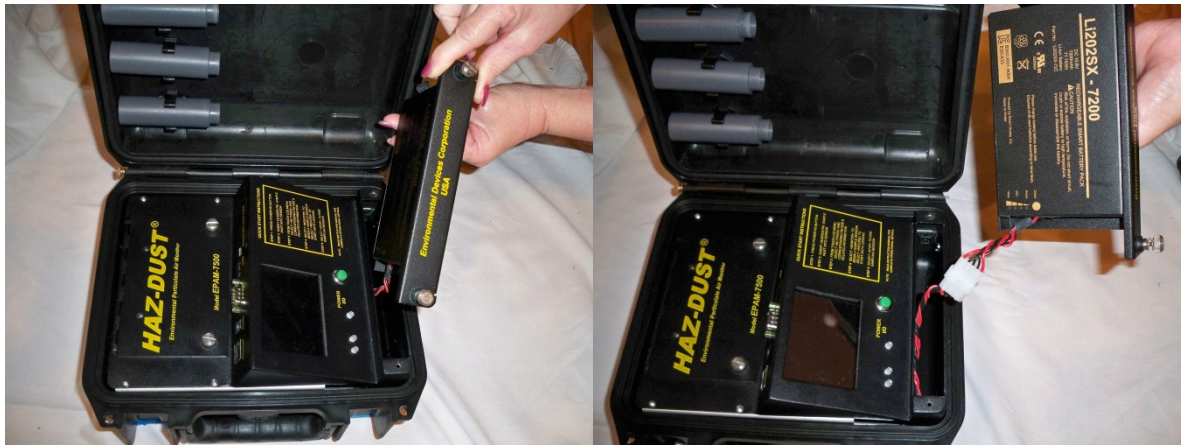
Figure 5-3. Diagram of battery being removed from Haz-Dust.
