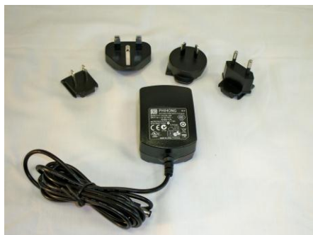
Figure 2-2: Universal transformer for 110V and 220V
