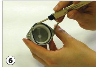
Remove O-ring from outlet plate.
