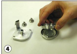
Lift accelerator plate A off collector plate.
