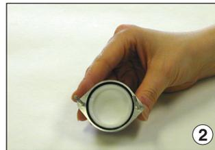
Insert 37-mm after-filter in outlet plate.
