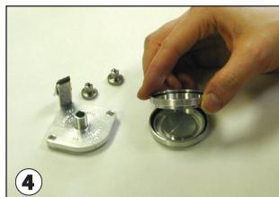
Lift accelerator plate A off collector plate.
