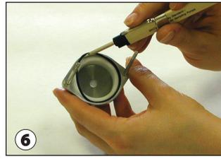
Remove O-ring from outlet plate.
