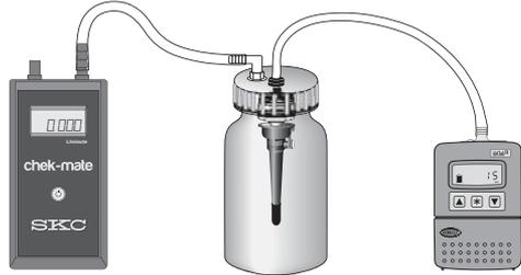
Figure 3. Calibration Train with Jar
