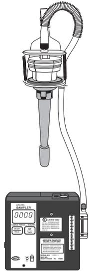
*Figure 2. DPM Sampling Train with GS-1 Cyclone, Cassette Holder, and Universal PCXR4 Pump*
