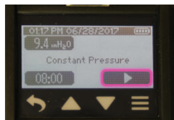
> Touch Run button in Advanced Menu to run pump in constant pressure.
