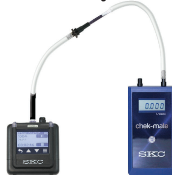
Figure 3. Single-tube Flow Verification Train Overview
