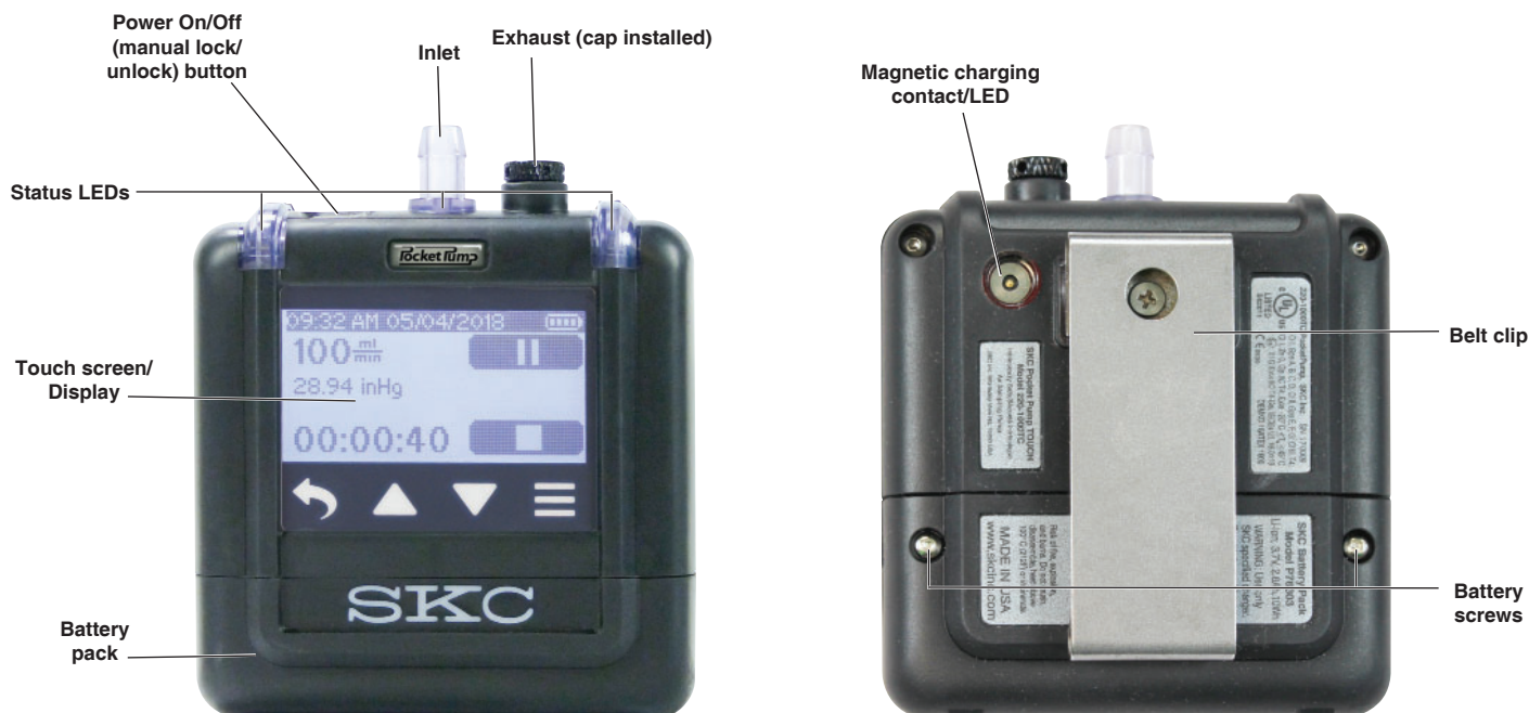
Figure 1. Pocket Pump TOUCH Physical Feature Overview
