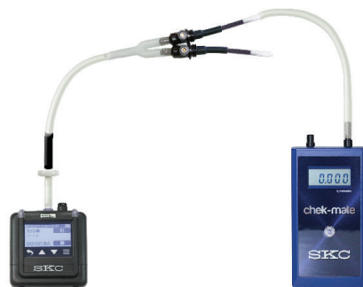
Figure 4. Multiple-tube Flow Rate Verification Train Overview - Constant Flow
