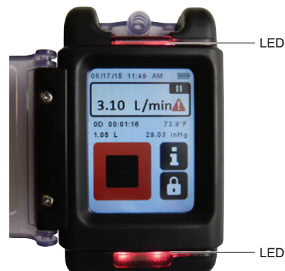
Figure 6. Red, flashing = Flow fault
