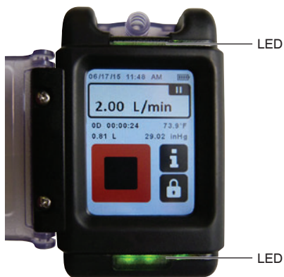
Figure 5. Green, flashing = Pump or schedule running
