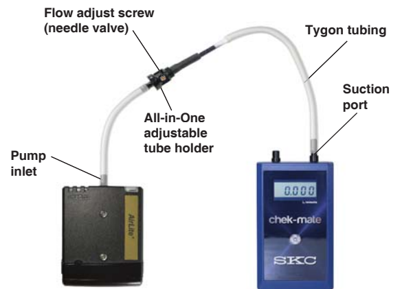
Calibration train with All-in-One connected to AirLite
