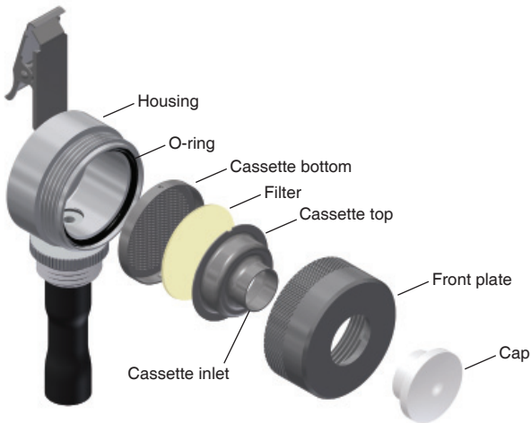
Figure 2. Configuration of Sampling Head and Filter Cassette
