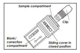
For Prefilled ULTRA: Write the sample stop time on the pouch label. Measure and record ambient temperature and atmospheric pressure and include in information sent to the laboratory. Ensure ID number on sampler matches ID number on pouch and place sealed sampler in resealable pouch.
