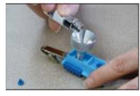
When sampling is completed, slide sampler cover to closed position.
