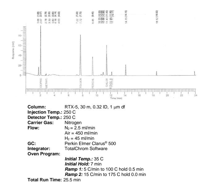
Figure 2. Sample Chromatogram – VOCs on Tenax TA Sorbent
