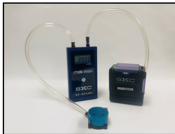
Figure 3. Jarless flow rate verification train
