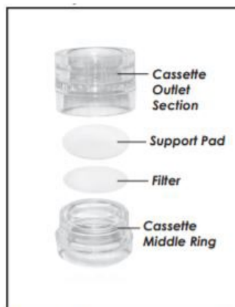
Figure 1. Assemble filter cassette for installation on cyclone
