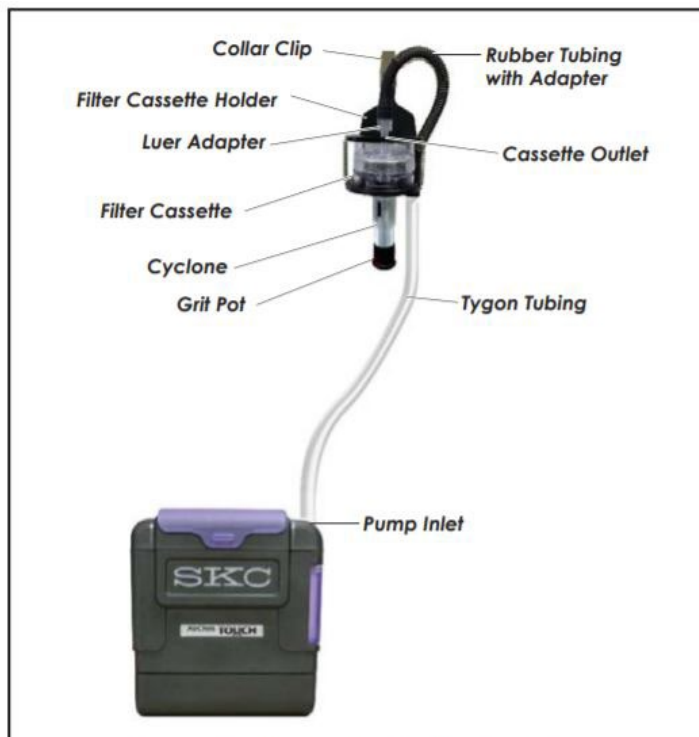
Figure 3. Sampling train with filter cassette and Aluminum Cyclone in Filter Cassette Holder
