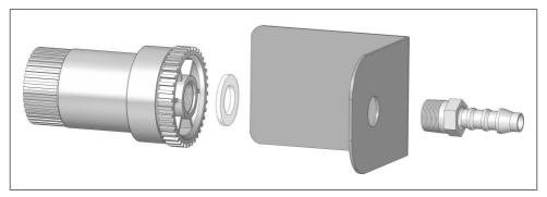
7. Screw the threaded hole on the asbestos sampling head onto the male thread at the top of the sampling mast.
