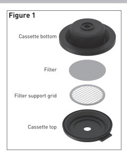
Place the metal filter support grid into the top part of the cassette. Place the filter to be used for calibration onto the support grid.
