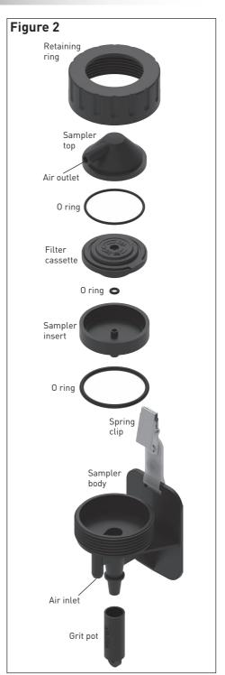
the cassette. Fit the retaining ring over the sampler top and screw down firmly to secure the cassette within the sampler and seal the cassette inlet and outlet.
