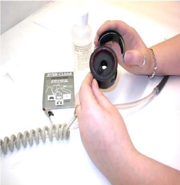
Figure 5-3. Removing the sensor cover.
