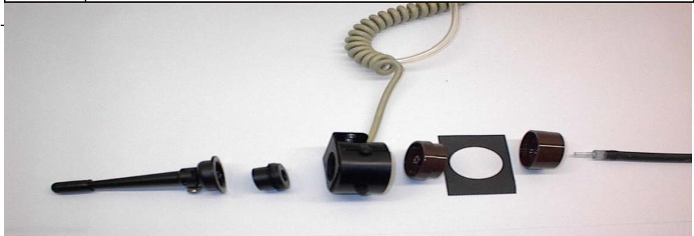
Figure 3.3. Component identifications from left to right: SKC GS-Cyclone for Respirable sampling, GSA-202 adapter, sensor head, disassembled filter cassette, filter, and air intake tubing.
