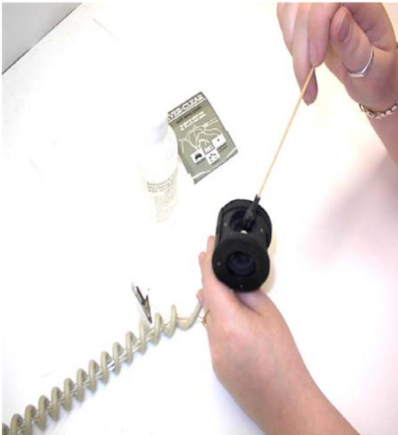
Figure 5-6. Sensor head being cleaned with cotton swab.
