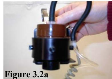
Figure 3-2 and 3-2a. Thoracic Inlet, sensor head, disassembled filter cassette, 37 mm filter, and air intake tubing. Optical sensor mounted on lapel bracket.
