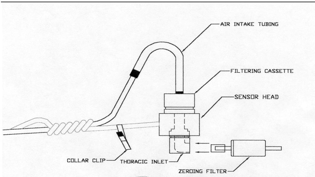
Figure 3-6. Diagram of zeroing filter being inserted into the Thoracic sampling inlet. This procedure is used for both Thoracic and Inhalable dust particles.
