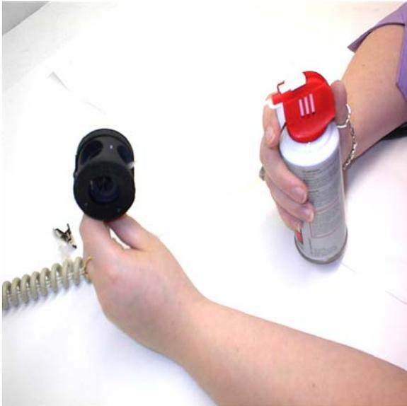
Figure 5-4. Dust being removed with low pressure air.
