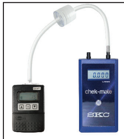
Flow rate verification train with filter cassette
