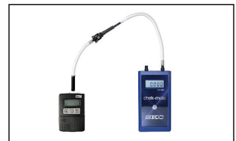
Flow rate verification train with All-in-One
