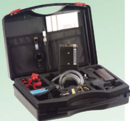
Dust sampling kit with IOM and Sidekick pump.
